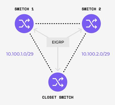
In this design, each L3 link is assigned a /29 network block. A /29 is a block of eight addresses, six being actually usable. In our example, the link to switch 1 has a range 10.100.1.0-7, where IP addresses 1 through 6 can actually be used.
